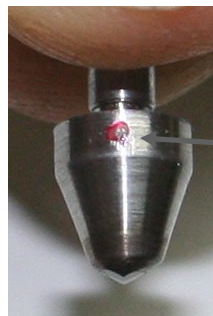
After loading indenter - run a sample indent to properly set the indenter
